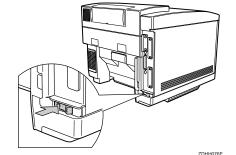
Check that the printer's power switch is set to the Off position (not depressed).
