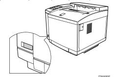
Attach the power cord to the socket on the back side of the printer.
