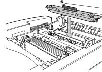
Turn the lock levers to hold the oil bottle and fuser cleaner
